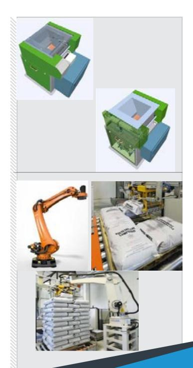
"We offer automated Polyolefin packaging from Bulk Railcars to 25KG or 50LB bags at a daily max capacity of 500 tons."
